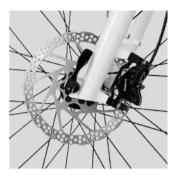
**DISC BRAKES** Highly responsive and easy to modulate hydraulic brakes, ideal for all weather conditions.
