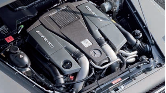
AMG 5.5-liter V8 biturbo engine
